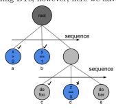
Figure 3: Behaviour Tree featuring two sequence nodes. The Tree is traversed top to bottom, left to right creating a priority order for horizontal traversal and a vertical hierarchical structure.
