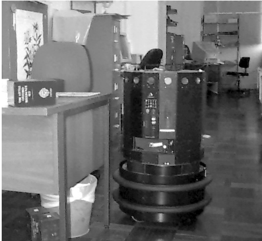
Figure 4.1: The Nomad 200 robot, of the Edinburgh Laboratory for Cognitive Neuroscience and Intelligent Systems. In this picture it is encountering a desk. The desk's surface is too low for the sonar sensors (the circles at the top of the robot's tower) to detect when proximate, and the legs too dark for the infra-red sensors (the lights at the base of the same tower) to detect. Consequently, the robot must learn about the desk with its bump sensors (the two rings around the robot's base).
